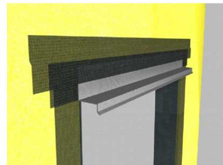
Overlap AquaFlash System over flashing leg minimum 51 mm (2 in).
