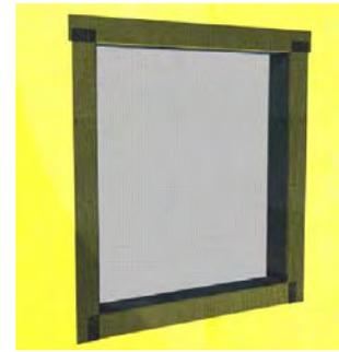
9. After the AquaFlash System materials have dried, the window and associated flashings may be installed in accordance with the window manufacturer's installation instructions.
