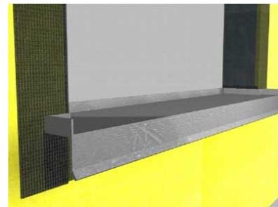
3. Clean the surface of the flashing as to be free of dirt, dust, oils or other contaminants that may interfere with adhesion.
