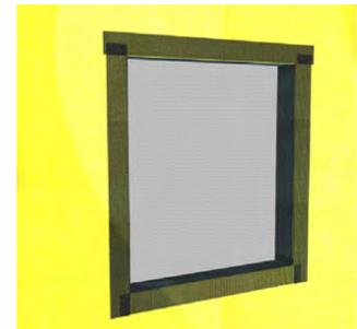
2. Install associated flashing material to the opening or face of the wall as necessary using appropriate corrosion resistant fasteners.
